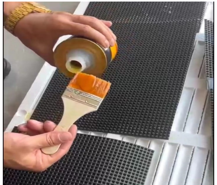
2- Glue is poured on the back of the edge of the mat using a brush
