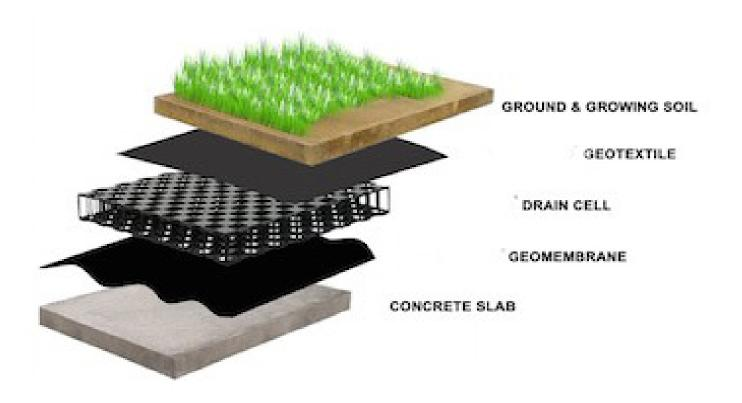
In our extensive range of geosynthetic products, we also manufacture premium geo drain cells/drainage mats, available in varying sizes.
